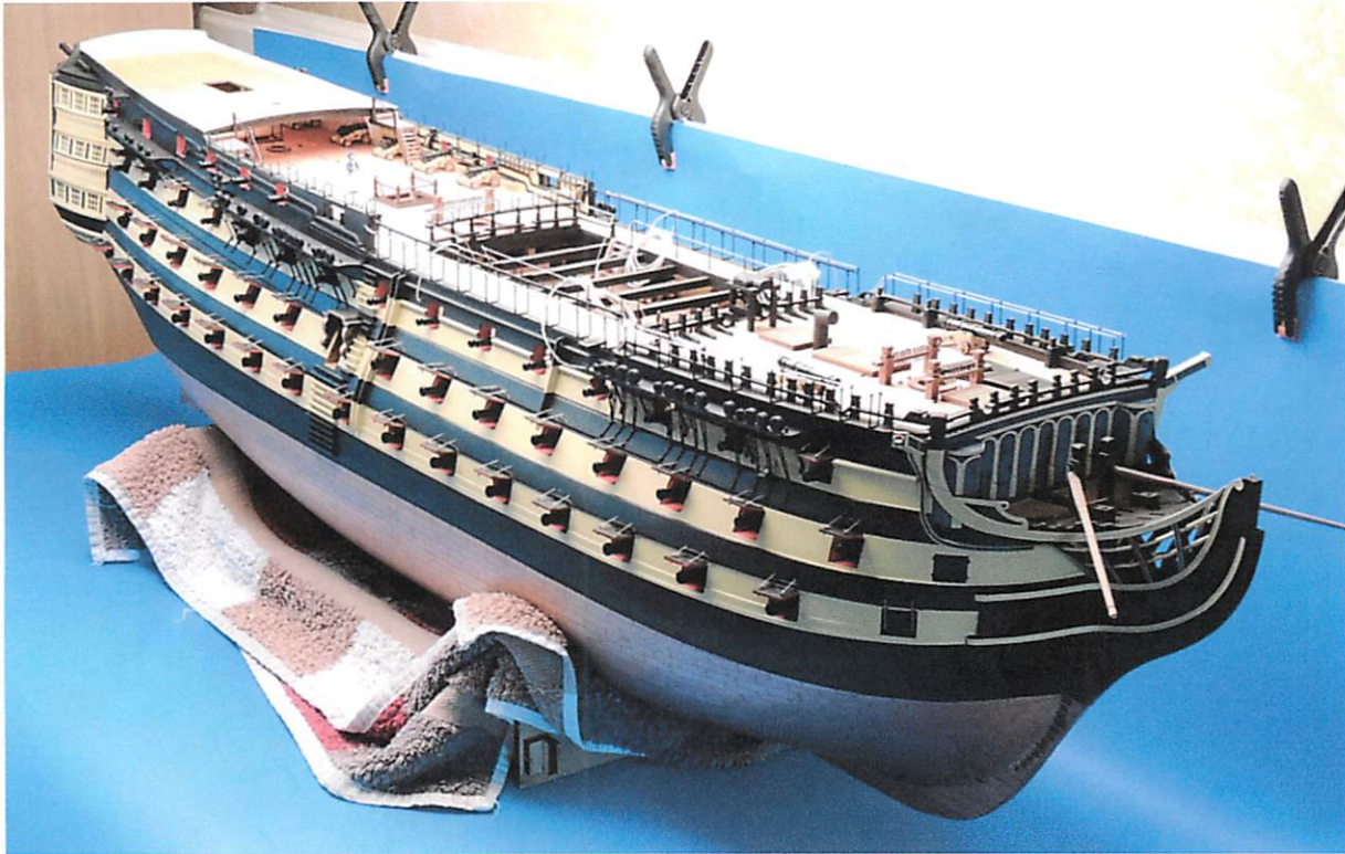
(Above) Boomkins dry fitted before painting. Because I used sources that show the bow platform deck at upper gun deck height, and not raised, the lower rail ekeing has a sharper curve due to the lower position of the platform, compared to as she looks now.
