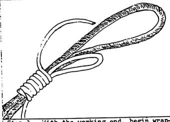
Step 3. With the working end, begin wrapping. Keep the coils close together. Keep count of the number of turns so later siezes are the same size.
