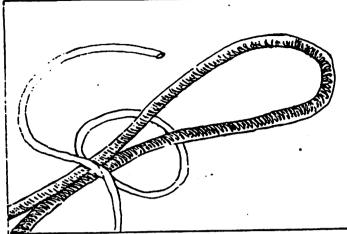
Step 1. Make aloop in the line to be siezed. Tie an overhand knot with the siezing line, leaving enough line to work with later.
