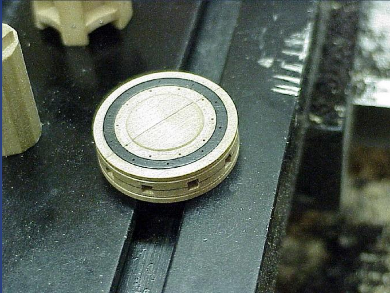
Holes drilled for reinforcing ring and pins for capstan bar retaining pins
