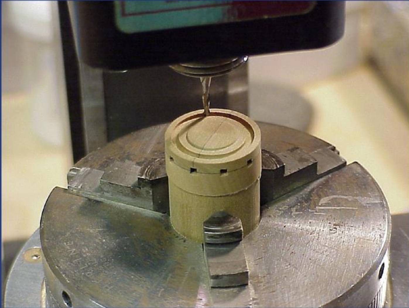
Milling recess for the iron reinforcing ring
