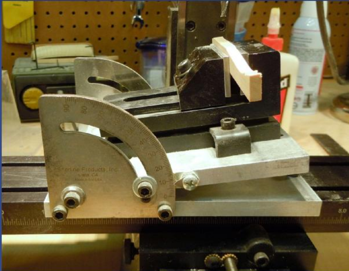
Mill with angle plate attached, 8° bevel cut
